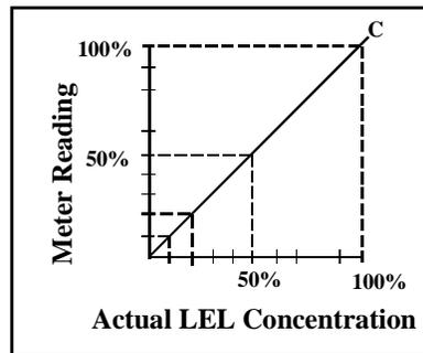
**Figure 1 Linear response to the gas used in the calibration**
