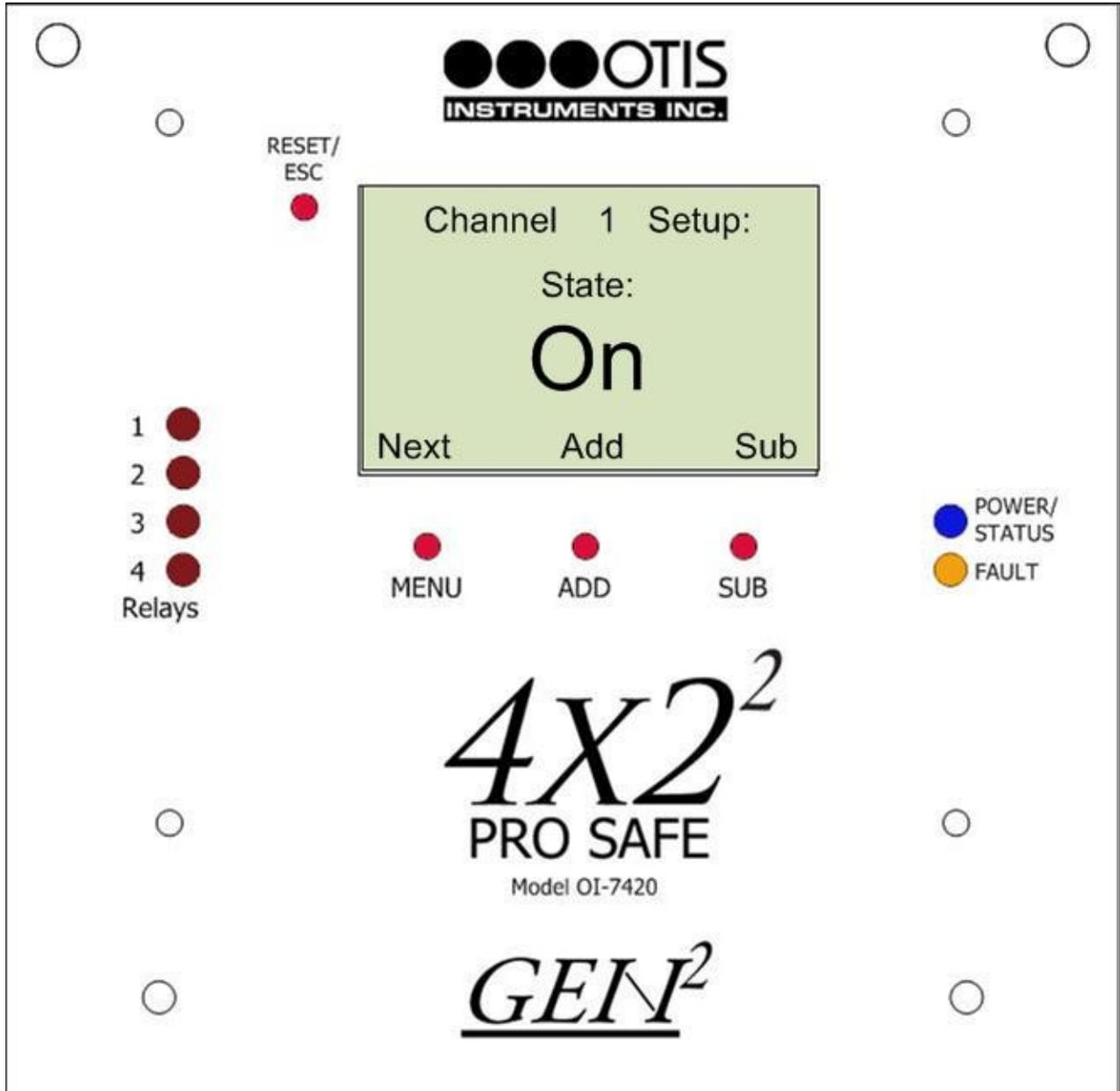
*NOTE: All channels must be setup as On/Off before the information screen is available. If the channel is set to “On”, additional settings will be available to set. If the channel is set to “Off”, there will be no additional settings available for that channel, and pressing MENU will allow the user to move to the next channel to be set to On/Off. Once both channels are set, press MENU once more to view System Information (see page 37).*
