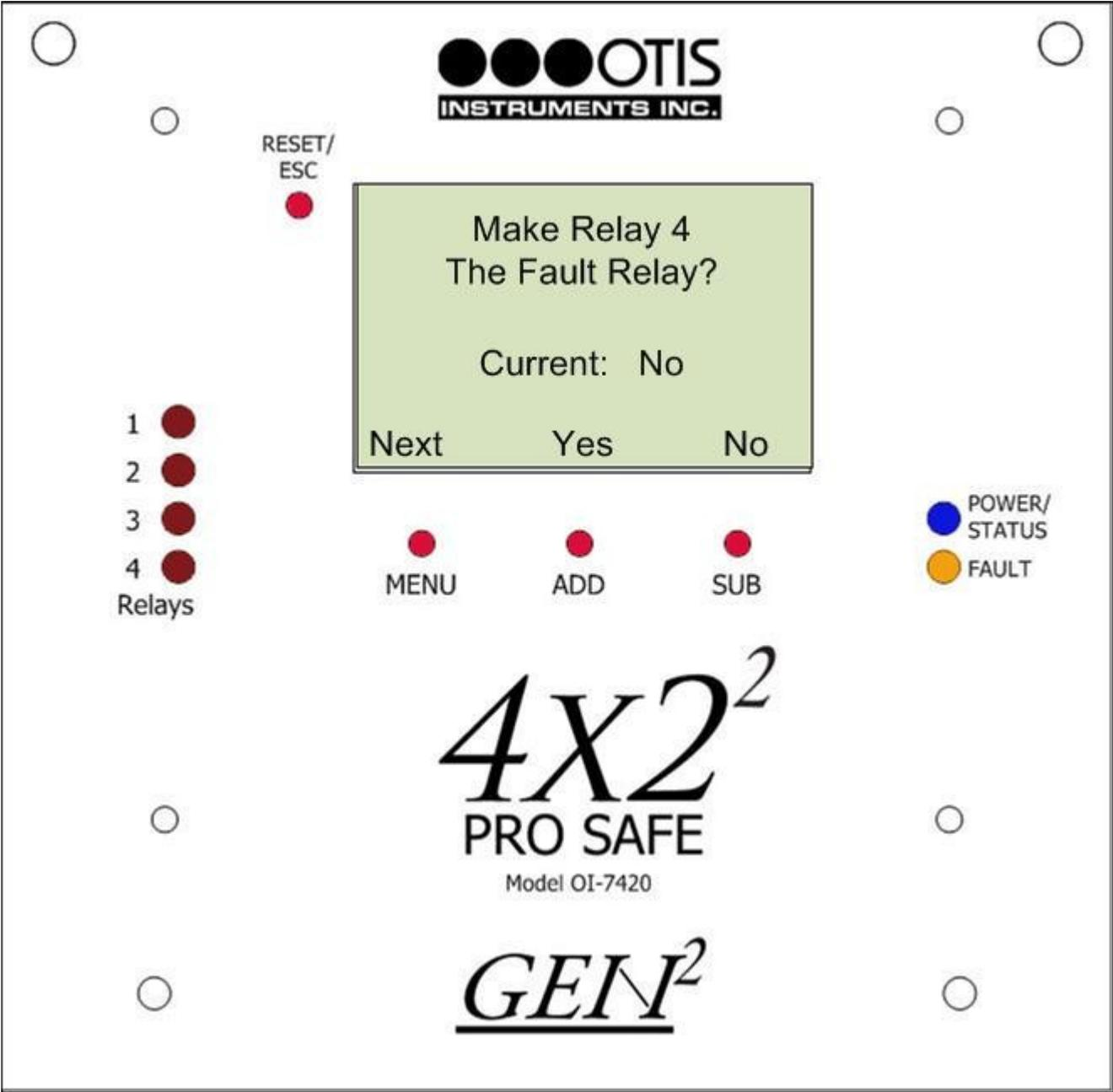
**Fault Relay Setup: Latching or Unlatching**
