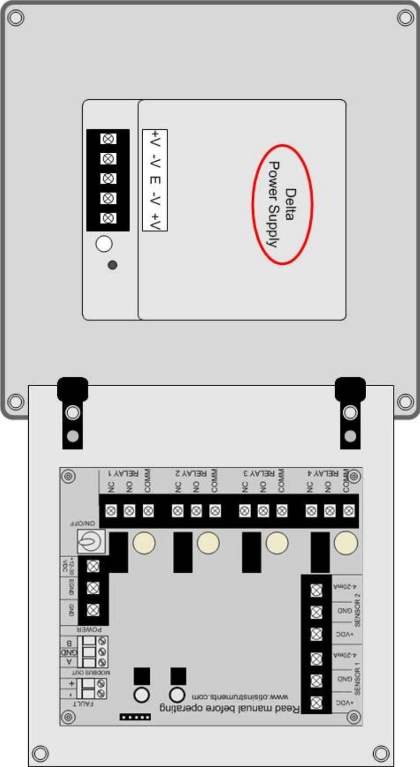
6. Connect a negative (black) wire from the Power Terminal terminal labeled “GND” on the Terminal Board.
