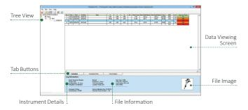
The HAVex meter is supplied with the Vibdata Lite software which allows you to download your measurements via USB for analysis and storage of data as required by the regulations. It is also possible to upgrade to Vibdata Pro which has the following added features:
