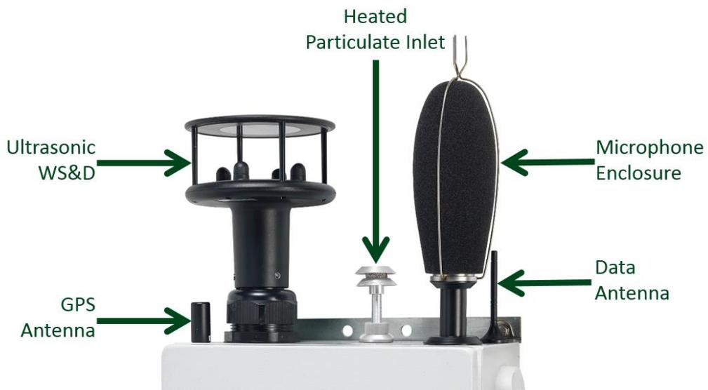
**Notes:** The GPS antenna supplied may be different to the one pictured above. The vibration sensor is not shown in the picture above as it is situated outside of the main Guardian2 enclosure.
