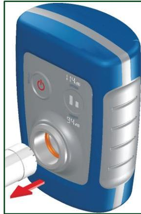
**Note:** Do not twist or screw on or off the calibrator on the microphone capsule.
