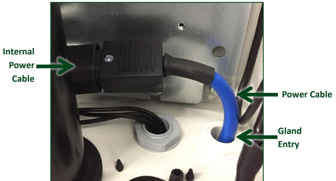
Once the cable has been fed through the gland to the outside, connect the correct plug as applicable. The 110VAC (coloured yellow) cable is supplied with the Guardian2 as standard. The 240VAC cable (coloured blue) is optional at the time of ordering and is supplied with a UK standard 3 pin plug.
