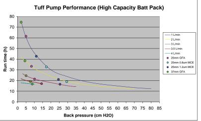
The **TUFF** pump incorporates a proven efficient double acting diaphragm pump mechanism with precise digital control. This offers the user excellent real time flow control and stability across a wide range of sampling media.
