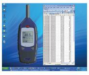
spreadsheet applications. Data stored within the CEL-246 can also be accessed since these meters act like a memory stick, allowing transfer of data to spreadsheet applications.
