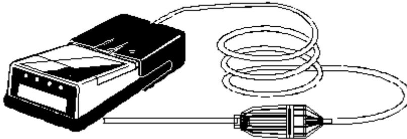
**Figure 1.5. Motorized sample-draw pump attached to detector**
