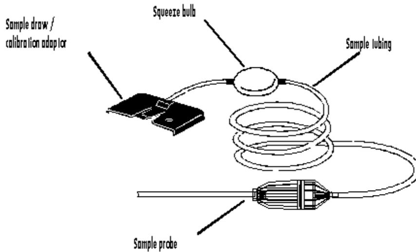
**Figure 1.1. Hand-aspirated (squeeze-bulb) sample-draw kit**
