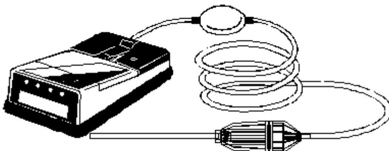
**Figure 1.3. Hand-aspirated sample-draw kit attached to detector**
