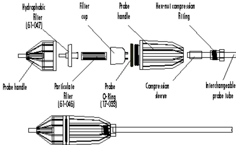
**Figure 1.2. Sample probe assembly**
