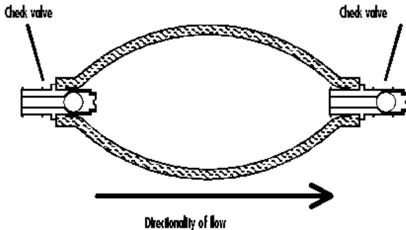
**Figure 2.1. Squeeze-bulb from manual sample-draw kit**
