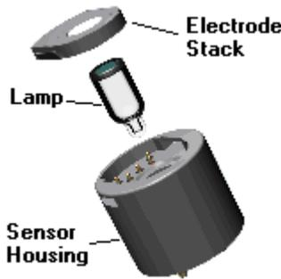
A special tool (Sperian part number 05-1365) is used to remove the electrode stack from the top of the sensor. This will allow access to the lamp.
