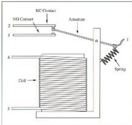
Diagram 1: Basic Structure of a single-pole-double-throw relay
