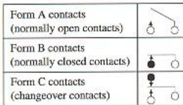
Diagram 3: Form A, B, and C Relays
