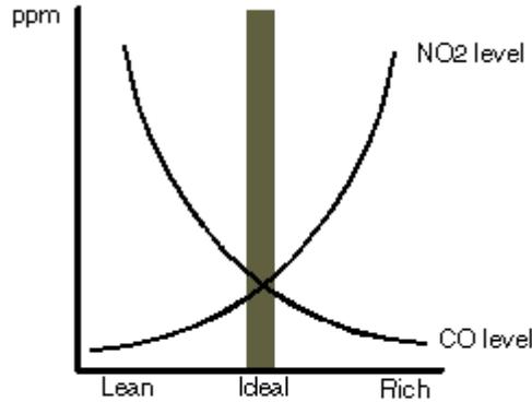
Figure 1: CO and NO<sub>2</sub> generation as a function of engine temperature
