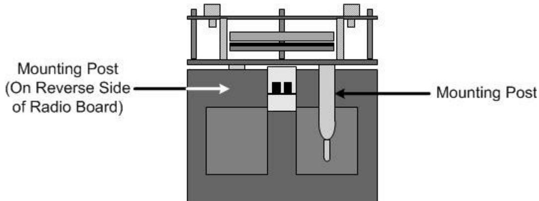
8. Verify that each mounting post is properly fitted in its corresponding eyelet inside the Moore enclosure.
