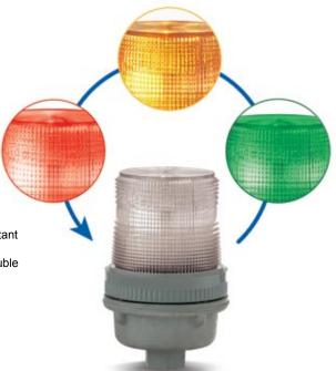
The Edwards 105XBRi Series XTRA-BRITE<sup>™</sup> LED Multi-Status Indicator is a heavy duty, reliable UL and cUL listed, multi-color visual signaling device. It features a corrosion resistant Type 4X enclosure that is UL listed for Marine use, and can be panel or conduit mounted. The base is manufactured from glass-reinforced thermoplastic polyester resin and the double fresnel lens is made of shatter resistant polycarbonate.
