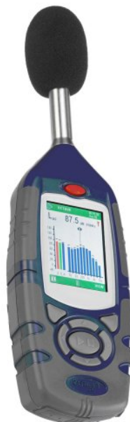
CEL-632.C Real time third octave band logging analyzer
